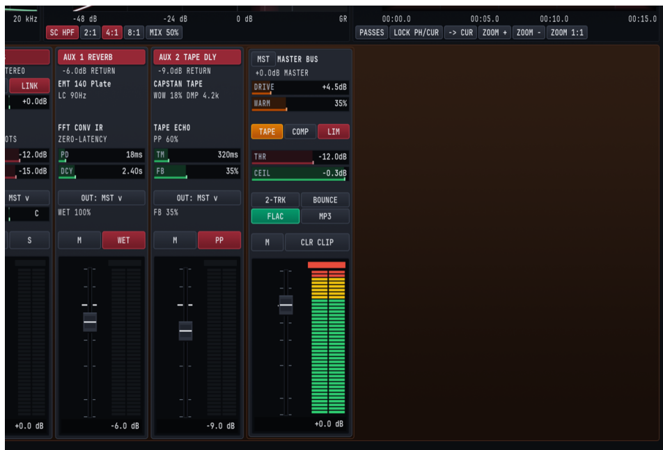
Figure 4.4: Subgroup Buses, Stereo Aux Returns, and the Master Bus strip on the right side of the Mix Console.
