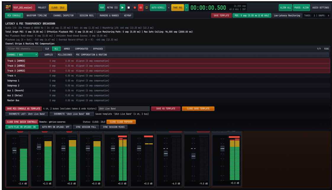
Figure 5.4: Plugin Delay Compensation (PDC) and Low-Latency Monitoring indicators in the Top Deck.
