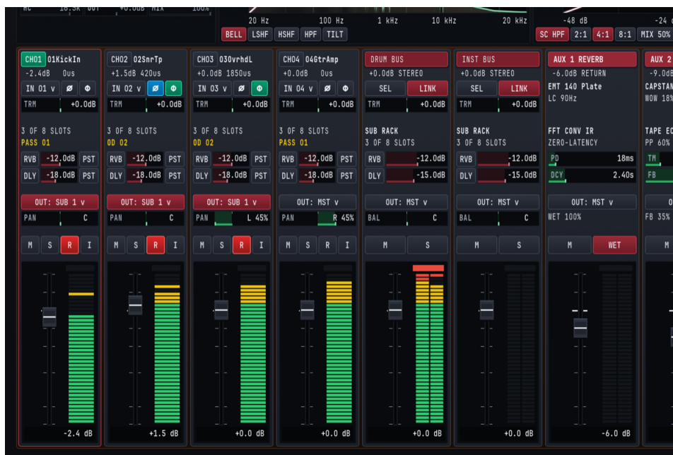
Figure 4.1: Input Track Channel Strips showing input routing, trim, phase badges, insert slot summaries, aux sends, output bus routing, and 40-segment meters.
