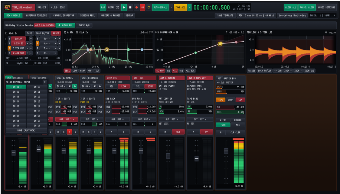
Figure 4.2: Selecting a physical audio input and routing buses on the Mix Console.
