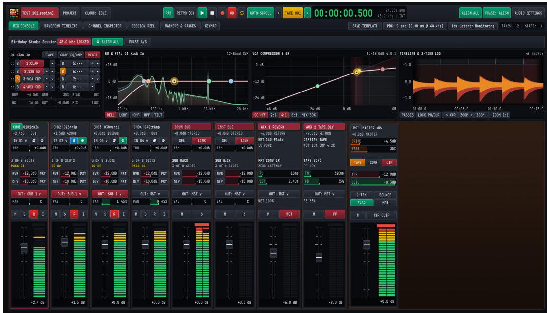
Figure 1.1: The Cave Recorder Mix Console workspace showing the Top Transport Deck, Upper Inspector Wells, and Lower Channel Strips.
